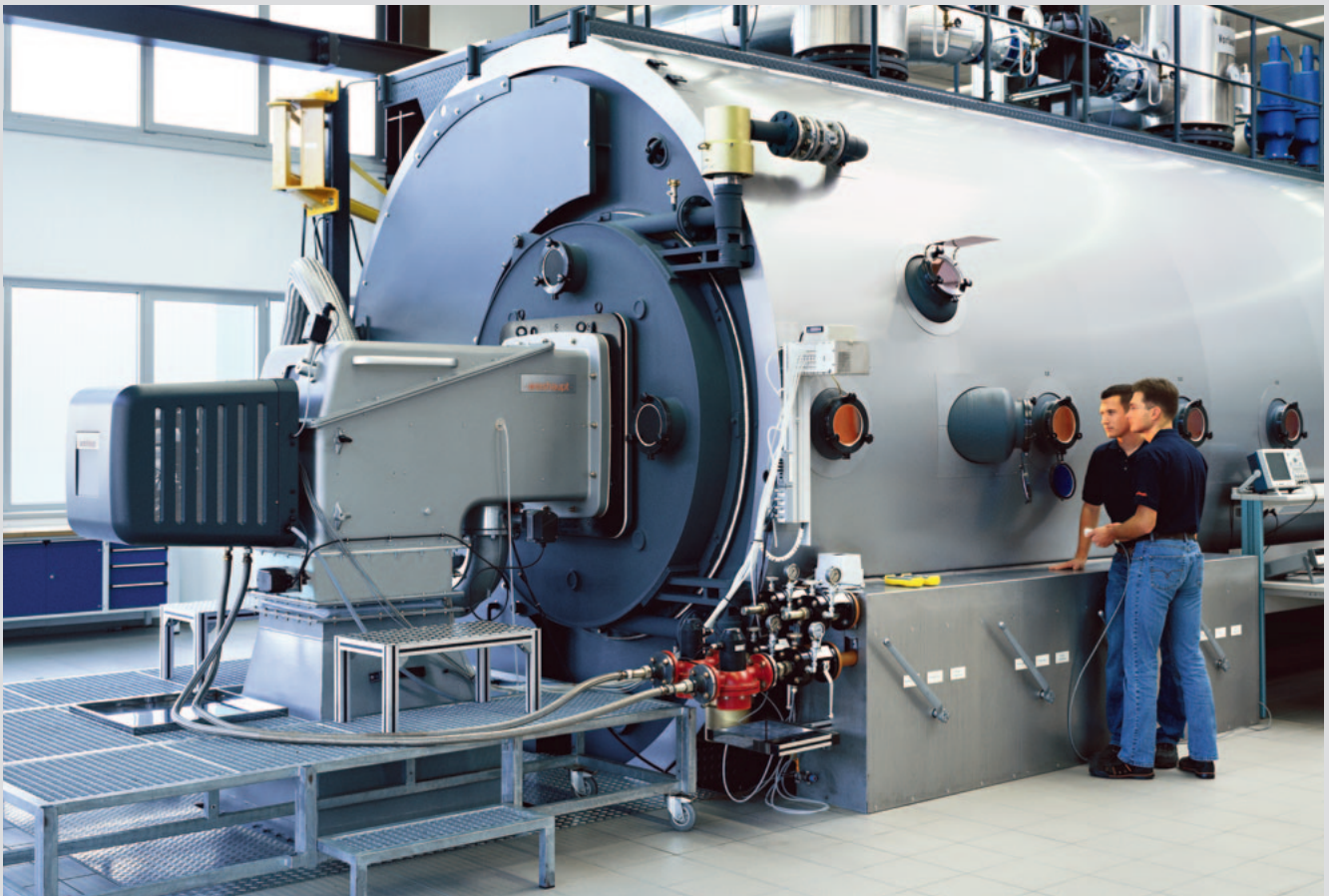
Burners rated up to 32 MW are tested on the world's largest test firing chamber in the R&D Centre
