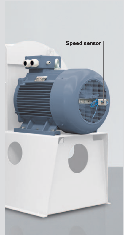
Fan motor with speed sensor for VSD
