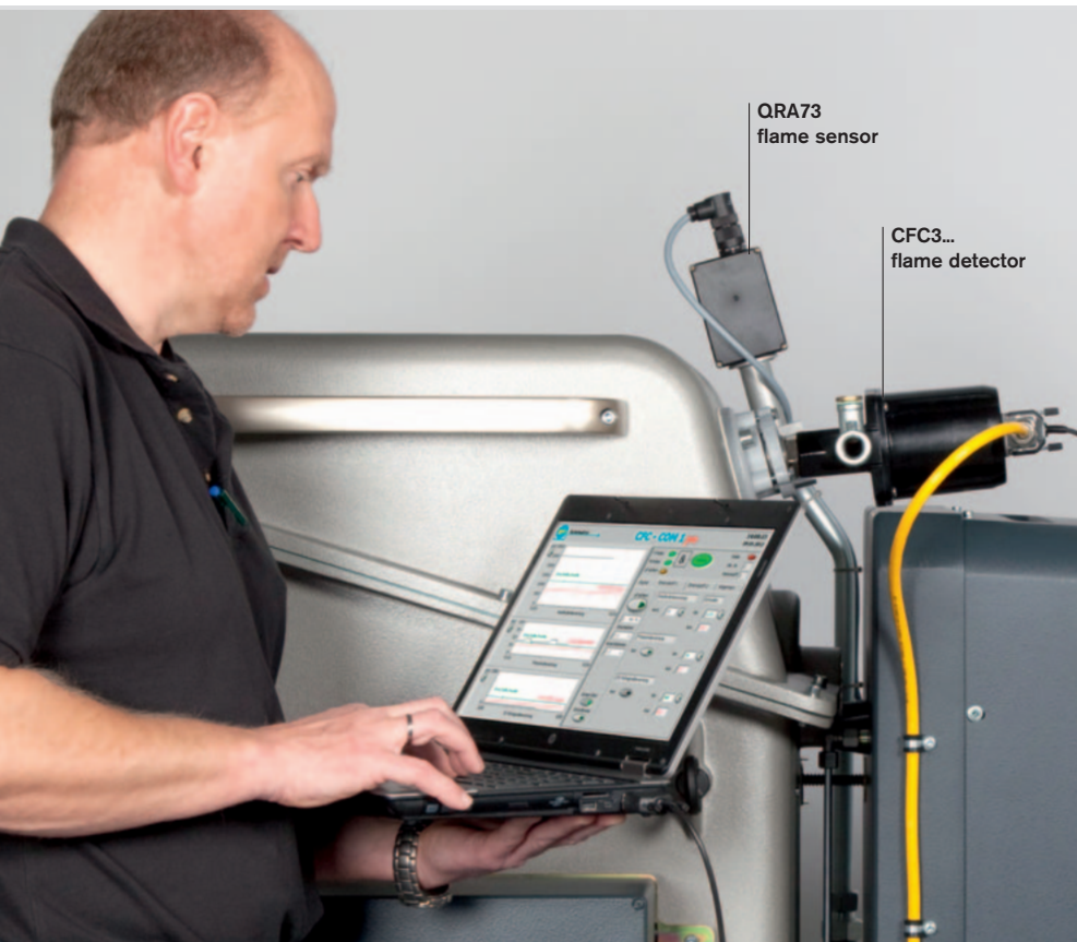
Testing and optimisation using a software tool
