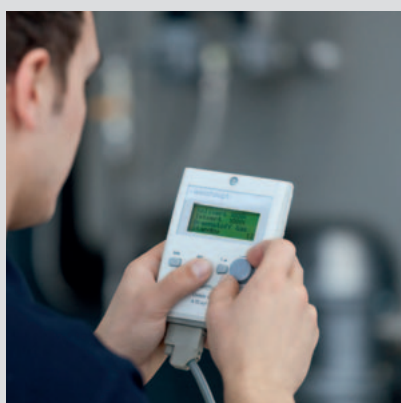
Setting via the ABE control and display unit
