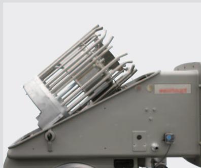
Mixing assembly in the servicing position
